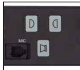
Radio rebroadcast switch & 2 x 10A rated switches for controlling external equipment e.g. lights.
